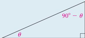
$$\begin{aligned}\sin \theta &= \cos (90^\circ - \theta), & \cos \theta &= \sin (90^\circ - \theta), \\ \tan \theta &= \cot (90^\circ - \theta), & \cot \theta &= \tan (90^\circ - \theta), \\ \sec \theta &= \csc (90^\circ - \theta), & \csc \theta &= \sec (90^\circ - \theta)\end{aligned}$$
